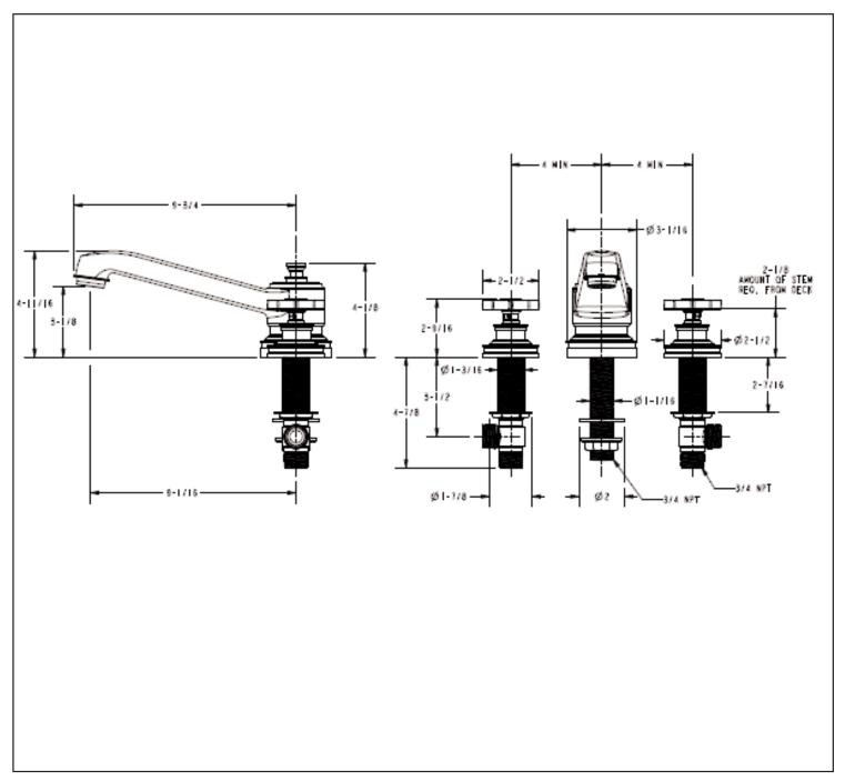
Recommended Deck Hole Size 1-1/4" Diameter Dimensions are in Inches and Approximation of a Typical Installation
