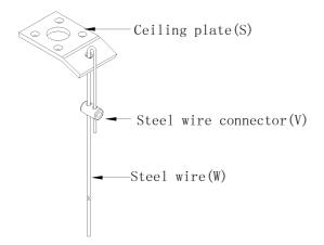
Pull the steel wire (W) to slide through one hole of the steel wire connector (V) and side hole of the ceiling plate (S). Then connect to the other hole of the steel wire connector (V).
