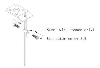
3. Using two connector screws (U), secure the steel wire connector (V) tightly based on desired hanging height.
