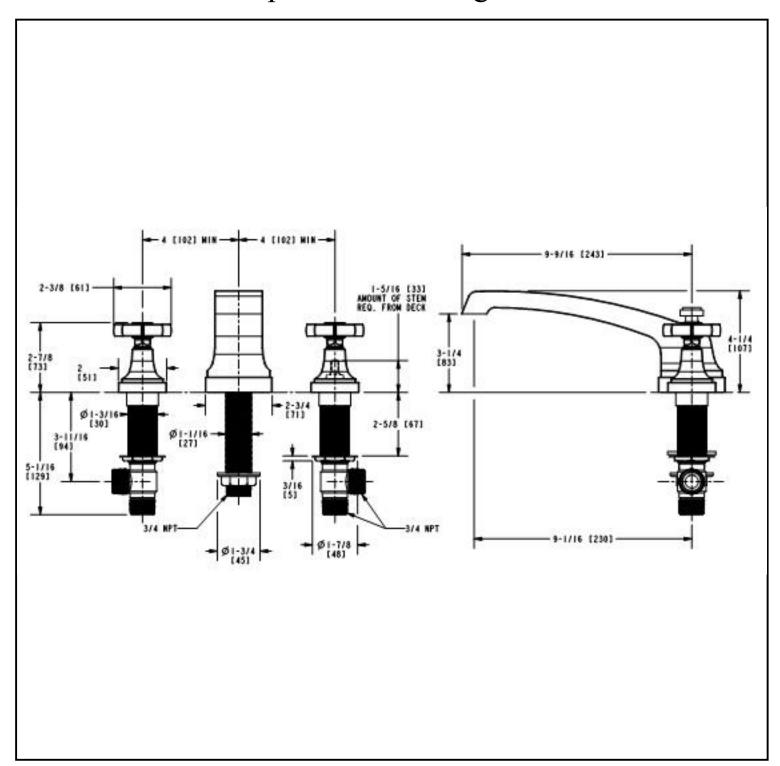
Recommended Deck Hole Size 1-3/8" Diameter Dimensions are in Inches and Approximation of a Typical Installation
