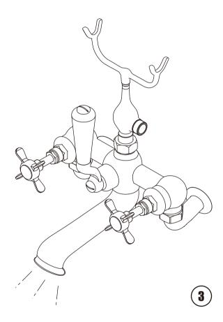
After installing faucet, open the hot and cold supplies to check for leaks. Turn on faucet handle for one minute to flush debris from faucet. Turn off the handle.
