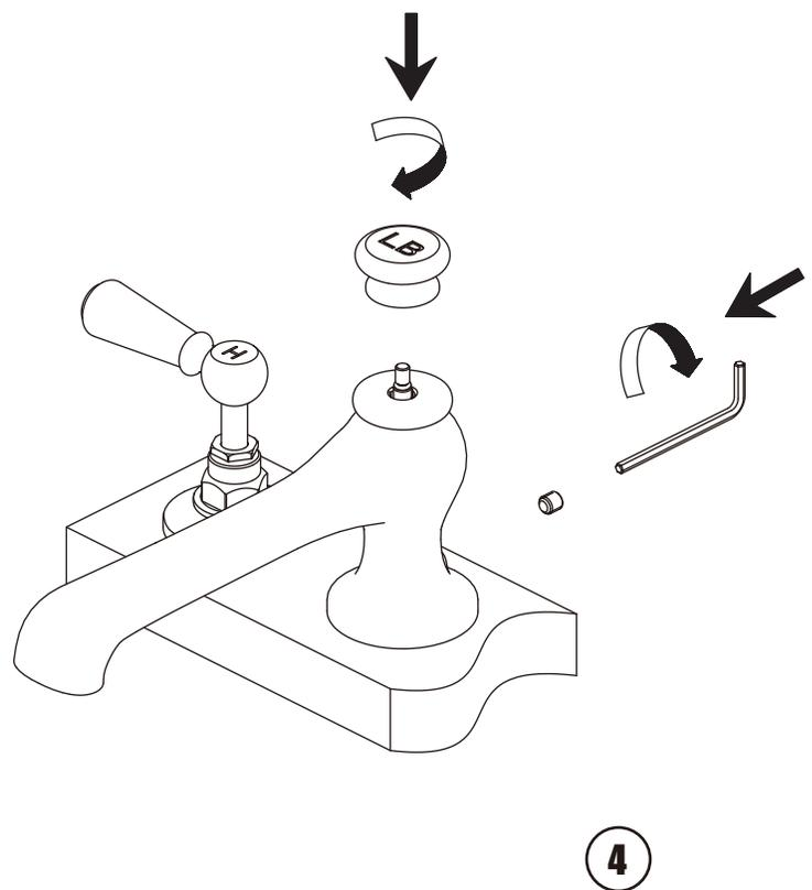
**4** Install the diverter knob. Finish installation by inserting set screw into access hole in back of spout and screw tightly.
