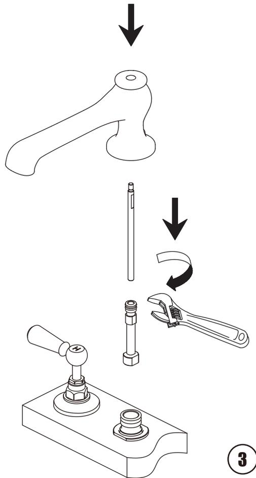
**3** Install the adaptor and diverter rod to the body and screw tightly. Place spout over spout hub.
