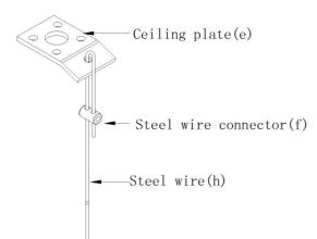
2. Pull the Steel Wire (h) to slide through one hole of the Steel Wire Connector (f) and side hole of the Ceiling Plate (e). Then connect to the other hole of the Steel Wire Connector (f).
