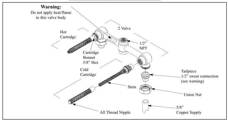
All thread connections are 1/2" NPT Dimensions are in inches and Approximation of a typical installation
