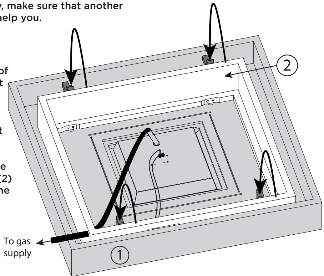
Secure the Table Base (2) to the Table Top (1) with four washers (B) and four screws (A) at the 4 supports.
