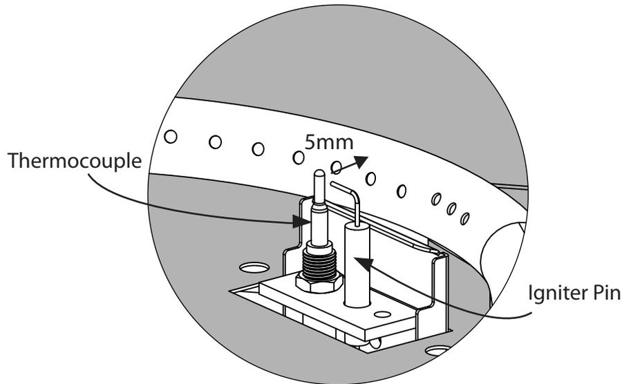
3. Make sure that the igniter pin and thermocouple are correctly positioned.
