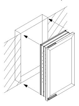
Mount cabinet by fastening the enclosed wood screws (B) to the inner side panels. Enclosed screws are to be used for installations into wood frames. For different wall material type additional screws / anchors may need to be purchased.
