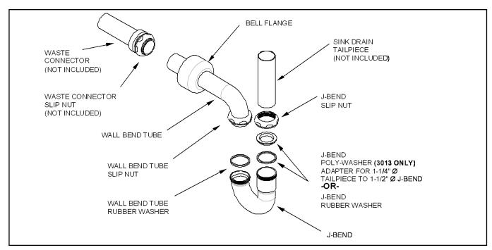
Hand tightening all the slide nuts should provide a good seal to joints
