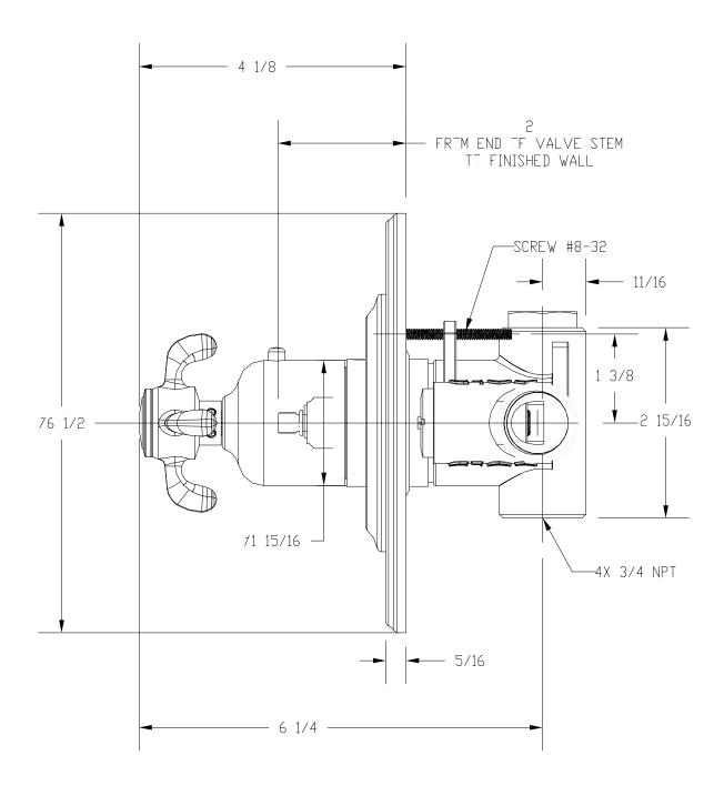
All Threaded Connections are 3/4" NPT Dimensions are in Inches and Approximation of a Typical Installation
