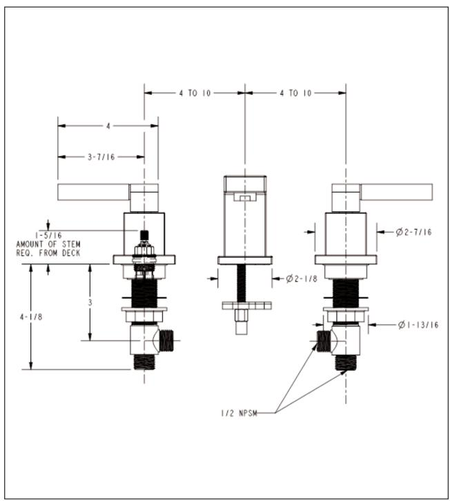
Recommended Deck Hole Size I-3/8" Diameter Dimensions are in Inches and Approximation of a Typical Installation
