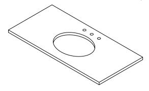
Inspect the Stone Top [A] for cracks or defects.
