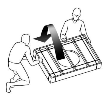
Carefully, without allowing any freefall, rotate the crate from vertical to flat.
