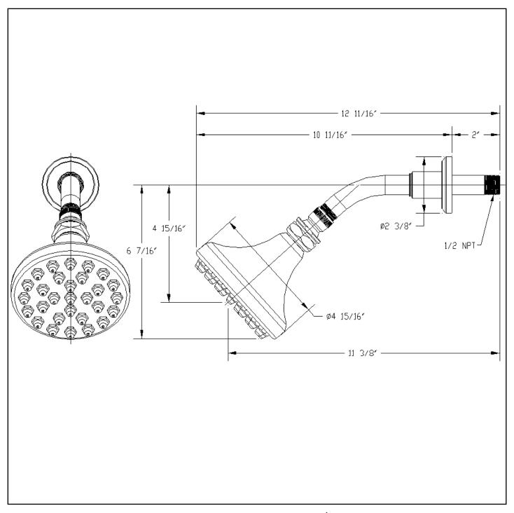
All Threaded Connections are <sup>1</sup>/<sub>2</sub>" NPT Dimensions are in Inches and Approximation of a Typical Installation
