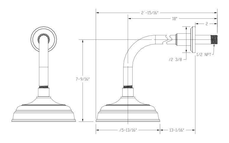
All Threaded Connections are <sup>1</sup>/<sub>2</sub>" NPT Dimensions are in Inches and Approximation of a Typical Installation
