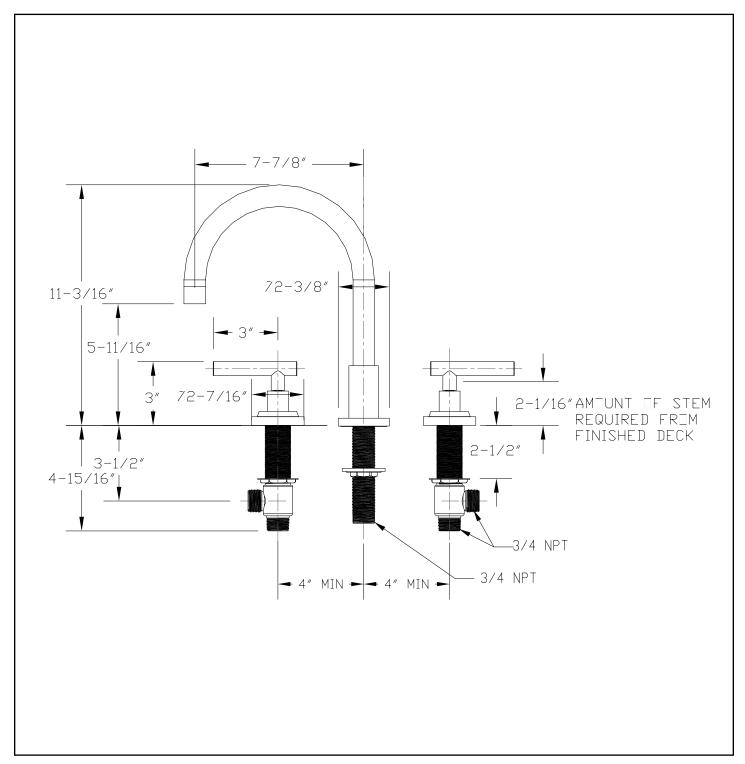
Recommended Deck Hole Size 1-1/4" Diameter Dimensions are in Inches and Approximation of a Typical Installation
