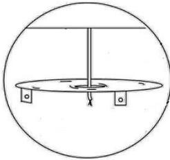
Place the top ceiling plate [A] flush against the ceiling, pull electrical cords through the hole and mark 4 anchor spots. Drill holes in the marked spots and place anchors in. **NOTE: Consult your local hardware store for proper anchors.**
