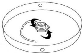
Use the plate nut wrench [I] to unscrew the two nuts holding the plate to the rod.
