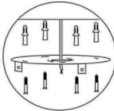
Pull wires protruding from the ceiling through the ceiling plate and screw the anchor screws in.
