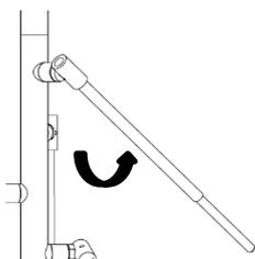
Turn the arm counterclockwise until it reaches the **recommended horizontal position**. Watch the sticker with arrows for the right direction. The recommended position is advisory only. Arms can be positioned pointing downwards or upwards.
