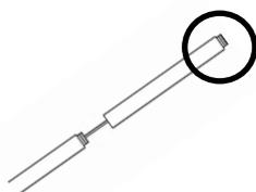
After removing the bottom ceiling plate [B], carefully pull the cords through selected extension rod(s) [E]. **NOTE: Make sure the rod is positioned with the thread upwards.**
