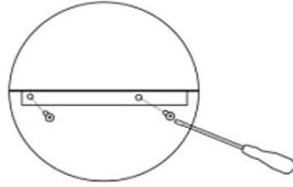
After removing the lamp frame from the box, use a flat-head screwdriver to unscrew 4 bolts [D] holding the ceiling plate.
