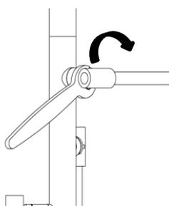
Use the wrench to turn the lock back clockwise. **NOTE: DO NOT force the lock. Turn gently until the arm is stable. Risk of breaking the lock!** Carry on downwards until all arms are positioned correctly.
