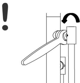
Use the arm wrench [H] to loosen the arm's lock. Turn the lock gently half a turn counterclockwise. **NOTE: DO NOT force arms without loosening the lock first.**
