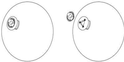
**NOTE: Included cotton gloves MUST be worn when handling glass globes.** Start mounting glass globes from the top arm downwards by first removing a plastic stopper from the globe to be mounted.
