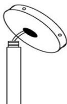
Pull the cords through the bottom ceiling plate [B] and screw it back on the rod with two nuts using the wrench [I]. **NOTE: Make sure the cord endings are not frayed. If yes, twist them back together.** Connect the cords back to the transformer terminal. (See Step 5 for reference)
