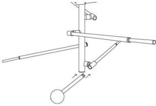
Mount arm counterweights [F] by screwing them onto each arm. **NOTE: To keep the balance of the lamp, mount weights on opposite pairs.**
