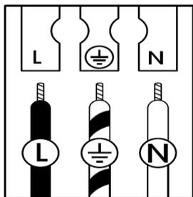
Junction boxes may vary depending on location. The diagram on the left shows the most common markings and manner of connecting the cords. **NOTE: We recommend installation by a licensed electrician.**
