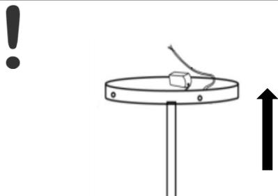
Lift the fixture up and hold under the top ceiling plate [A] to make electrical connections. **NOTE: TWO PEOPLE are needed for this and the three following steps.**
