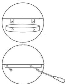
Lift the bottom ceiling plate [B] flush with the top ceiling plate [A] and line up the bolt holes. Use a flat-head screwdriver to screw four bolts [D] in.
