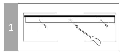
NOTE: HEAVY ELEMENT. HANDLE WITH CARE. After removing the lamp frame from the box, use a flat head screwdriver to unscrew 6 bolts [D] holding the ceiling plate.
