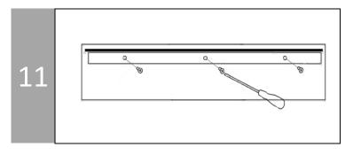
Lift the bottom ceiling plate [B] flush with the top ceiling plate [A] and line up the bolt holes. Use a flat-head screwdriver to screw four bolts [D] in.
