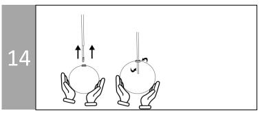
Carefully mount each globe onto the arm tip and screw it on.
