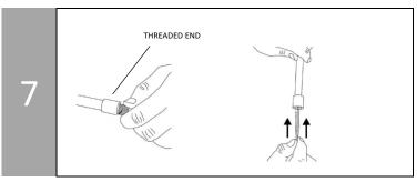
After removing the plate [B], unscrew the threaded inserts from the lamp rods. Carefully pull the cords through selected extension rods [E]. **NOTE: Make sure the rods are positioned with the thread upwards.** Screw the threaded inserts on top of extension rods.
