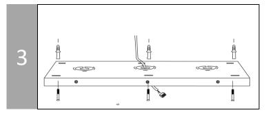
Pull wires protruding from the ceiling through the ceiling plate and screw the anchor screws in.
