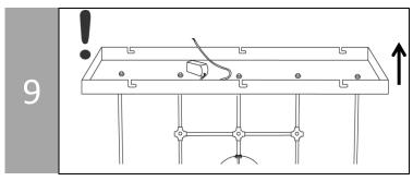
Lift the fixture up and hold under the top ceiling plate [A] to make electrical connections. **NOTE: TWO PEOPLE** are needed for this and the three following steps.
