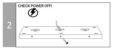
Place the top plate [A] flush against the ceiling, pull electrical cords through the hole and mark 6 anchor spots. Drill holes in the marked spots and place anchors in. NOTE: Consult your local hardware store for proper anchors.
