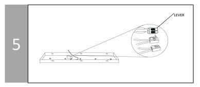
Disconnect the lamp cords by lifting the levers on the terminal and pulling out the cords.
