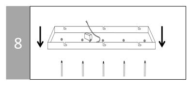
Pull the cords through the bottom ceiling plate [B] and screw it back on the rods with the nuts using the wrench [G]. **NOTE:** Make sure the cord endings are not frayed. If yes, twist them back together. Connect the cords back to the transformer terminal. (See Step 5 for reference)
