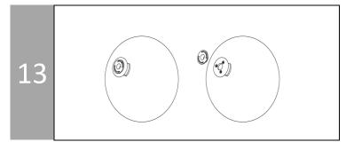
NOTE: Included cotton gloves MUST be worn when handling glass globes. Start mounting glass globes by first removing a plastic stopper from each globe to be mounted.
