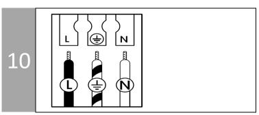
Junction boxes may vary depending on location. The diagram on the left shows the most common markings and manner of connecting the cords. **NOTE: We recommend installation by a licensed electrician.**
