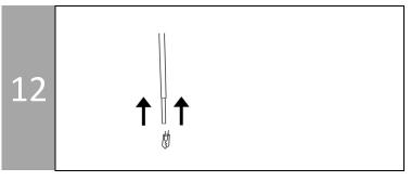
Carefully insert 7 included 1.6W LED G4 bulbs into slots on the tip of each arm.
