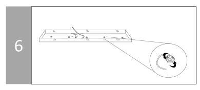
Use the large nut wrench [I] to unscrew the nuts holding the plate to the rods.
