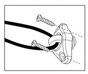
**Consider Position of Tension Device:** The tension device should be positioned on the window frame or the wall so that the tension device and control cord do not interfere with operation/hanging of drapery. Install tension device so that the cord is taut, without stretching or pulling down on it. Stretching the cord will cause excessive wear. Do not twist or cross the control cord.
