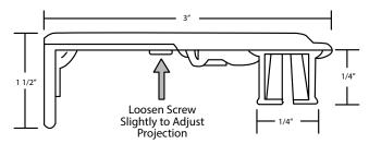
7. Once desired projection is set for all the brackets, lock the bracket into position by tightening the track depth adjustment set screw (see drawing below).
