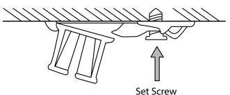
4. Tighten track set screws on all the brackets to secure track to brackets.
