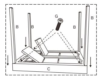
STEP 1: Insert the teak post (B) into the corner hole of the chaise. Pull up the chaise back, then screw in bolt (G) with Allen wrench (F). Repeat for each post.
