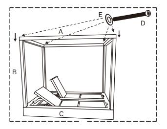
STEP 2: Place teak canopy top (A) on the teak posts (B), aligning the holes. Screw in bolts (D) with Allen wrench (F). Use aluminum pole (H) to attach canopy; see detail below.
