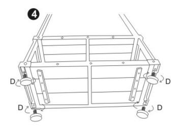
Place levelers (D) at the bottom of unit. Adjust as per floor level.
