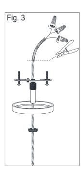
3. Cut the wires to desired height.
