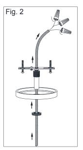
1. Remove set screw from mounting loop.
