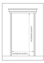
• Measure the interior widths, depths and heights of all elevator doors to be used for delivery.
