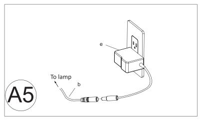
5. Plug the transformer cord into the upper body cord (B) and plug the transformer into your outlet.
