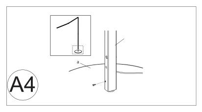
4. Insert the provided screw to secure the lower body to the base.
