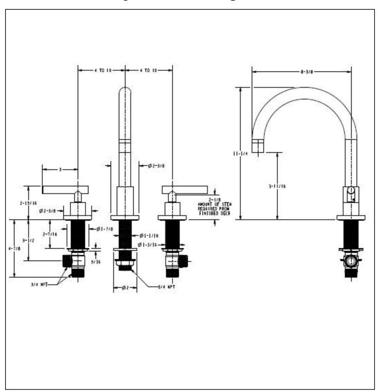
Recommended Deck Hole Size 1-5/16" Diameter Dimensions are in Inches and Approximation of a Typical Installation
