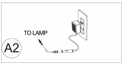
2. Plug the transformer into the wall. Insert the transformer's cord into the end of the lamp's cord.
