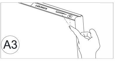
3. Press and hold the circle to change color between warm and cool. Adjust brightness by placing your finger along the touchstrip.
