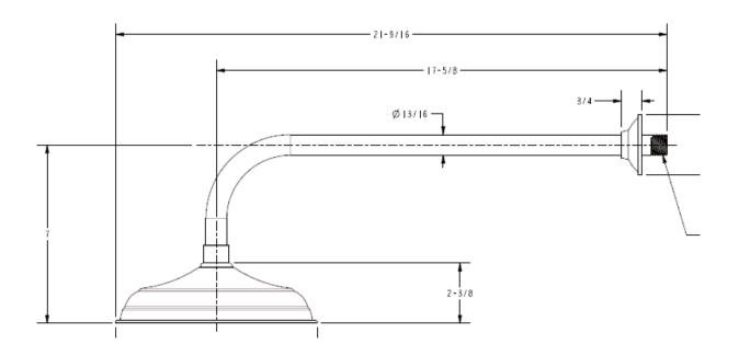
All Threaded Connections are <sup>1</sup>/<sub>2</sub>" NPT Dimensions are in Inches and Approximation of a Typical Installation
