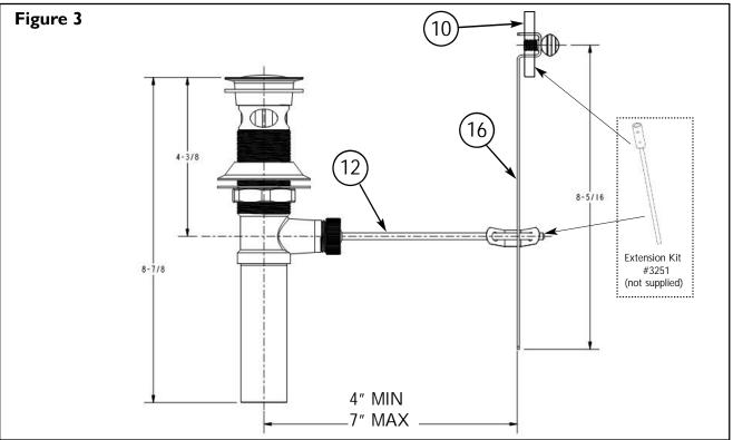
Note: Extension Kit (# 3251) for ball ROD (12) and/or pop-up ROD (10) available (sold separately). See Figure 3 for nominal dimensions. (Extension Kit connection must not interfere with CLIP (15), cutting item (12) and/or (10) may be required.)
