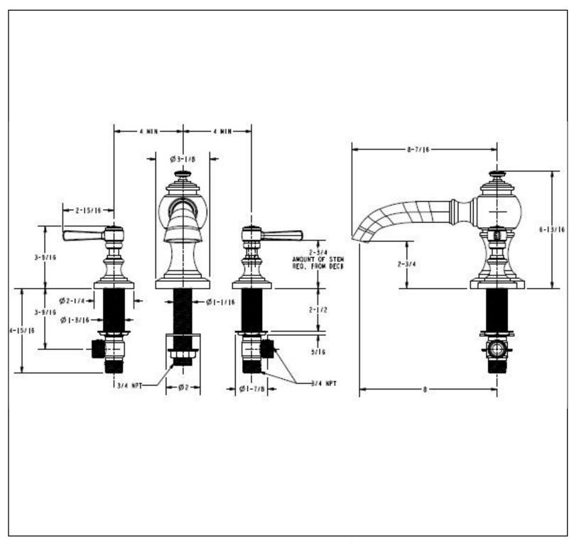
Recommended Deck Hole Size 1<sup>1</sup>/<sub>4</sub>" Diameter
