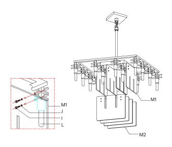
Figure 2: Installation for the middle of the outer part of the glass plates (M1 & N1). Install 2 pcs of M1 first, then fix 4 pcs of N1.
