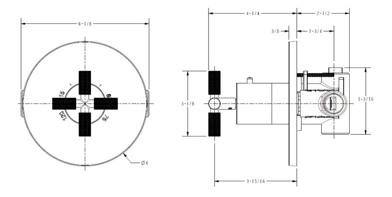
All Threaded Connections are 3/4" NPT Dimensions are in Inches and Approximation of a Typical Installation Technical support: 1-866-417-5207 Customer Service: 1-877-747-4671 RH-8944X REV -
