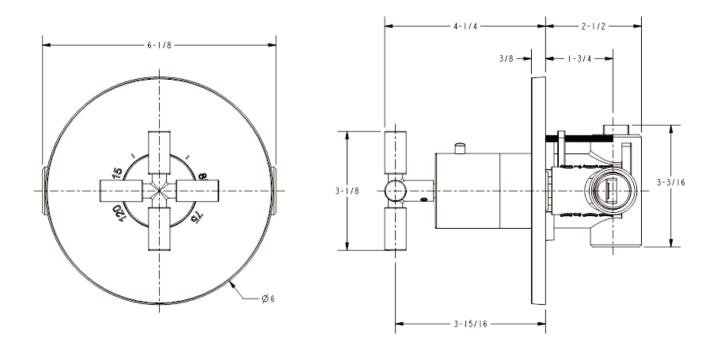
All Threaded Connections are 3/4" NPT Dimensions are in Inches and Approximation of a Typical Installation Technical support: I-866-417-5207 Customer Service: I-877-747-4671 RH-8844X REV -
