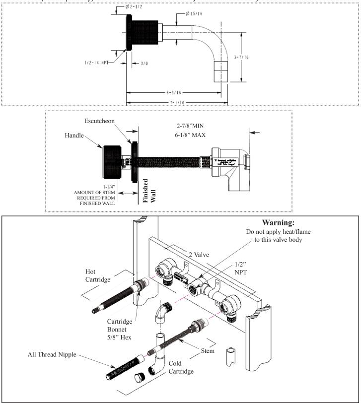
All thread connections are 1/2" NPT Dimensions are in inches and Approximation of a typical installation Technical support: 1-866-417-5207 Customer Service: 1-877-747-4671 RH-89
