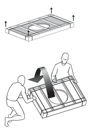
Remove metal bands, unscrew the slats or lid, and lift the Stone Top [ A ] out of the crate.
