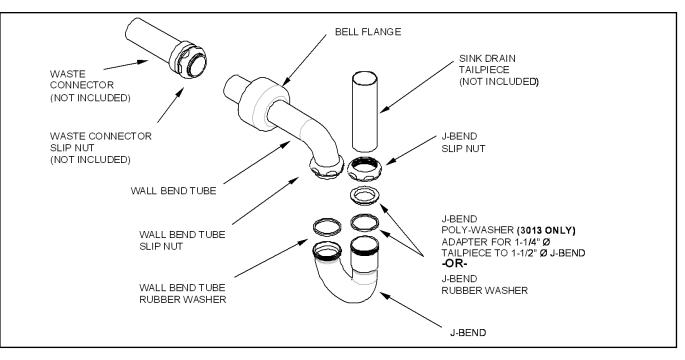
Hand tightening all the slide nuts should provide a good seal to joints **Contents:** (1) 1-1/4" J-bend, (1) 1-1/4" Wall bend, (2) 1-1/4" Slip nuts, (2) 1-1/4" Rubber washers, (1) Bell flange.
