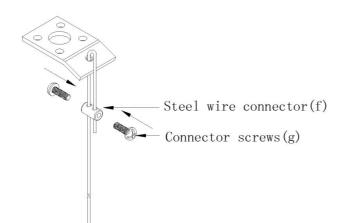
3. Using two Connector Screws (g), secure the Steel Wire Connector (f) tightly based on desired hanging height.
