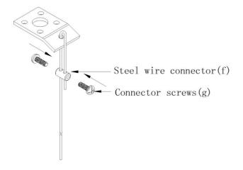
3. Using two Connector Screws (g), secure the Steel Wire Connector (f) tightly based on desired hanging height.
