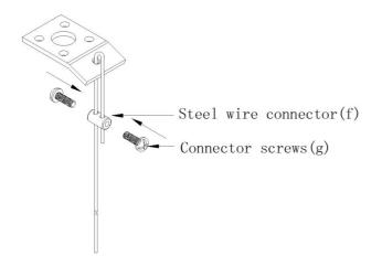
3. Using two Connector Screws (g), secure the Steel Wire Connector (f) tightly based on desired hanging height.
