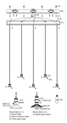
NOTE: you may shorten the hanging length of each cord by loosening the set screw on the fitting where the cord meets the canopy. Once you have set the desired length, retighten the set screw to lock the cord in place.
