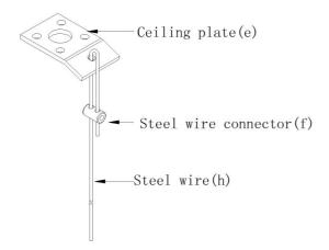
2. Pull the Steel Wire (h) to slide through one hole of the Steel Wire Connector (f) and side hole of the Ceiling Plate (e). Then connect to the other hole of the Steel Wire Connector (f).
