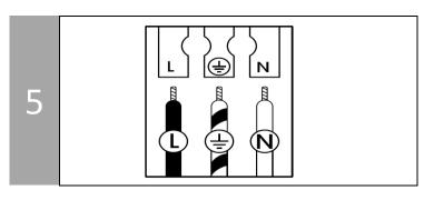
Junction boxes may vary depending on location. The diagram on the left shows the most common markings and manner of connecting the cords. **NOTE: We recommend installation by a licensed electrician.**
