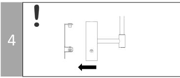
Move the sconce [B] towards the wall and hold near the wall plate [A] to make electrical connections.
