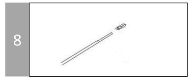
Carefully insert 1 included 1.6W LED G4 bulb into the slot on the tip of the arm.
