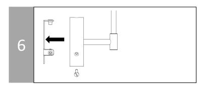
Move the sconce [B] flush with the wall plate [A] and line up the bolt holes. Use a flat screwdriver to screw three bolts [C] in.
