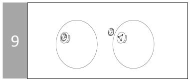
NOTE: Included cotton gloves MUST be worn when handling glass globes. Start mounting the glass by first removing a plastic stopper from the globe to be mounted.
