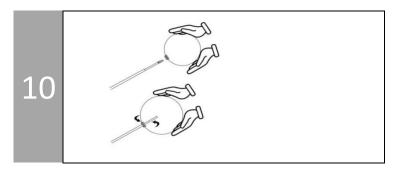
Carefully mount the globe onto the sconce tip and screw it on. The assembly is complete. Restore power and enjoy your Schwung Lamp.
