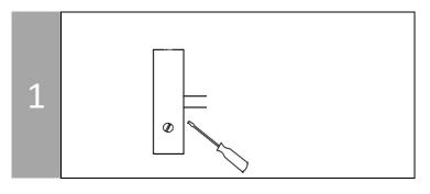
After removing the lamp frame from the box, use a flat head screwdriver to unscrew 3 bolts [C] holding the wall plate.
