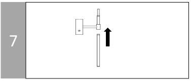
Screw the bottom tube [E] in. **NOTE: Do not** use force as it may cause thread damage.
