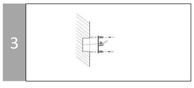
Pull wires protruding from the wall through the wall plate and screw the anchor screws in.
