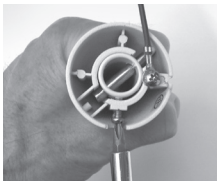
remove half-ball and stopper pin
