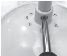
reinstall and tighten stopper screw
