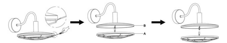
3. Unscrew the short-slotted screws, then carefully take out the LED panel from Cover (A).
