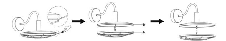
3. Unscrew the short-slotted screws, then carefully take out the LED panel from Cover (A).
