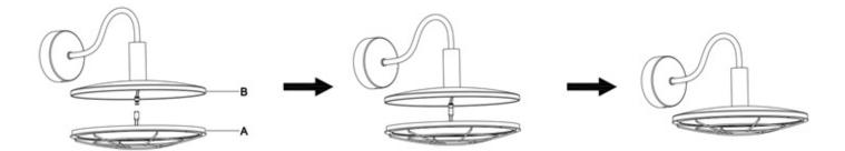
6. Secure Cover (A) to Cap (B) by screwing in the long-slotted screws.
