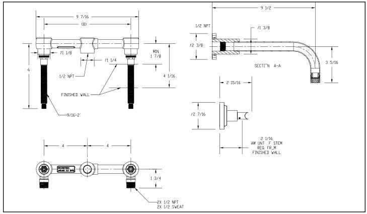
Dimensions are in Inches and Approximation of a Typical Installation
