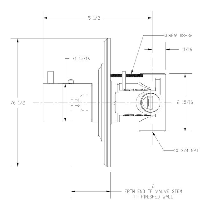
All Threaded Connections are 3/4" NPT Dimensions are in Inches and Approximation of a Typical Installation
