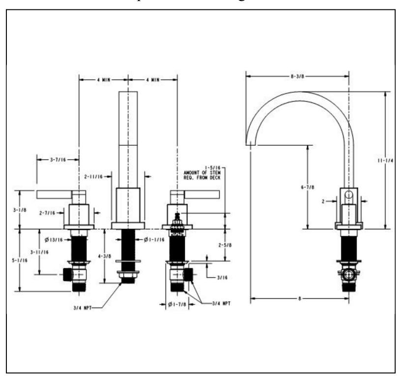
Recommended Deck Hole Size 1-1/4" Diameter Dimensions are in Inches and Approximation of a Typical Installation
