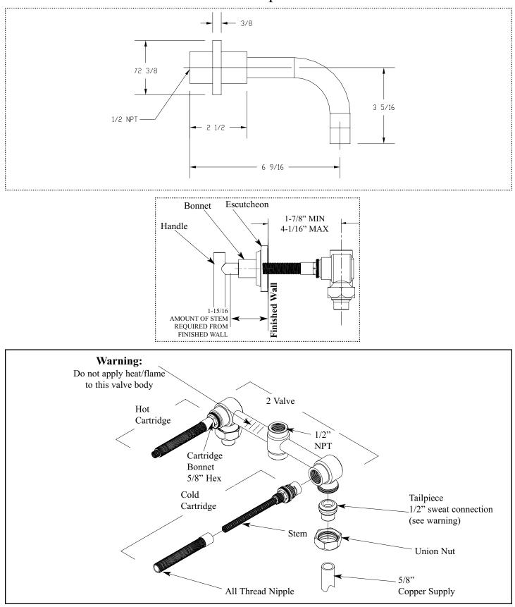
All thread connections are 1/2" NPT Dimensions are in inches and Approximation of a typical installation
