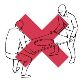
Do not carry Stone Top  $\,$  [A] horizontally as it increases the risk of breakage or cracking.
