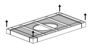
Remove metal bands, unscrew the slats or lid, and lift the Stone Top [ A ] out of the crate.
