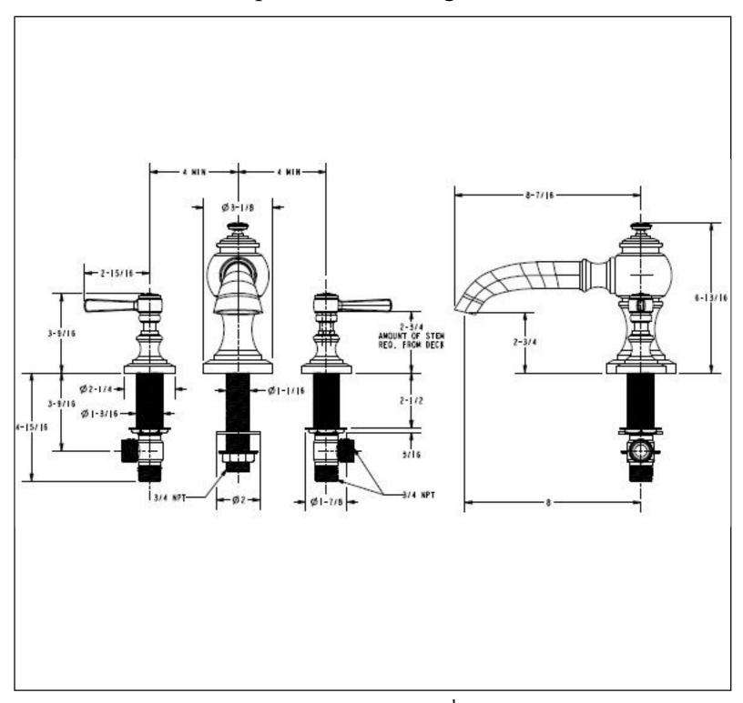
Recommended Deck Hole Size 1<sup>1</sup>/<sub>4</sub>" Diameter
